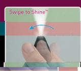
Features dual electrode capacitive sensing technology, which we call Swipe-To-Shine™
